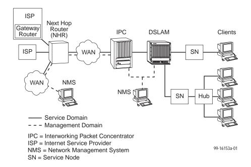
These procedures assume that Asynchronous Transfer Mode (ATM) is used on the link between the IPC and the next hop router (NHR).
